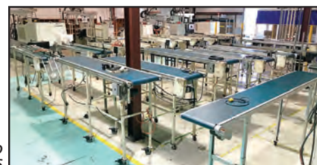
VIEW OF VARI-SPEED BELT CONVEYORS
