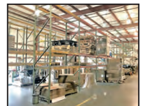
VIEW OF ADJUSTABLE PALLET RACKING
